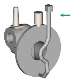
The initial methoding of the casting included two top feeders connected to the rim and boss section. Metal flow is controlled by a bottom gating system.
