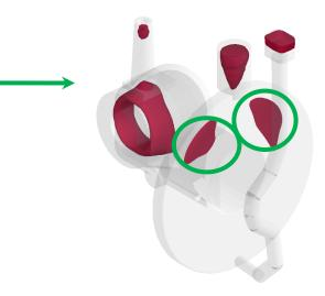
Solidification time analysis indicates presence of last to solidify region in the flange. These locations are matching with the location of defect observed on the shop floor.
