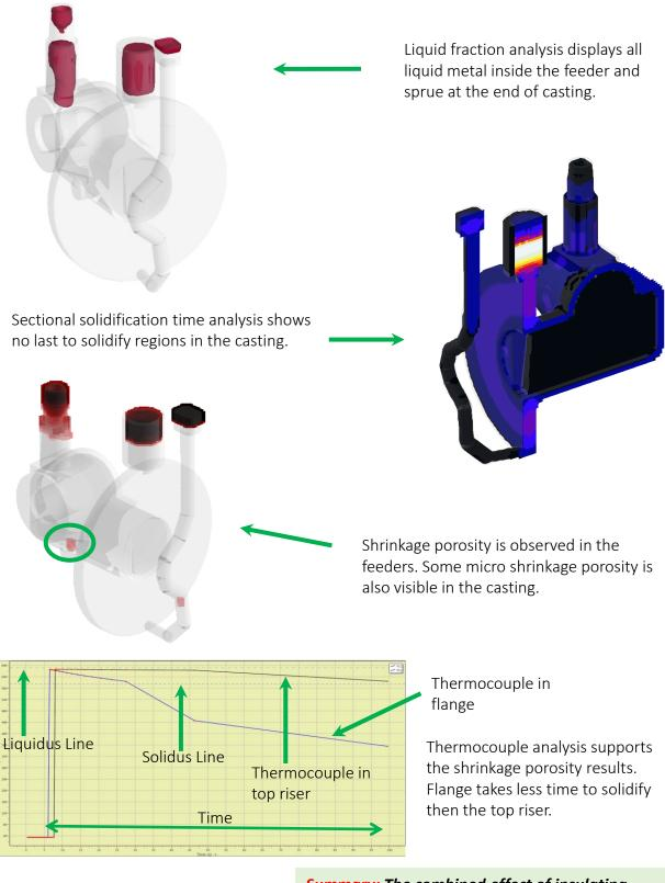
*Summary:* The combined effect of insulating sleeves and core chill reduced the rejections to less than half. Complete elimination requires changing the cavity orientation in the die.
